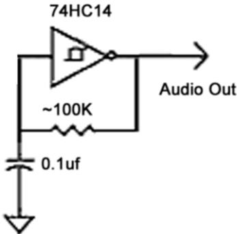
The schematic to the left shows a very simple audio oscillator that will be the starting point for our Theremin circuit. It produces a constant tone with a pitch determined by the resistor and capacitor. Larger values for either component will lower the pitch and smaller values will raise it.
